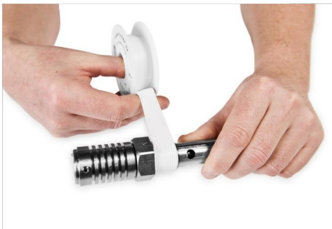
Apply Teflon or liquid gasket on sensors with a conical thread. For other thread types, solid gasket is used.
