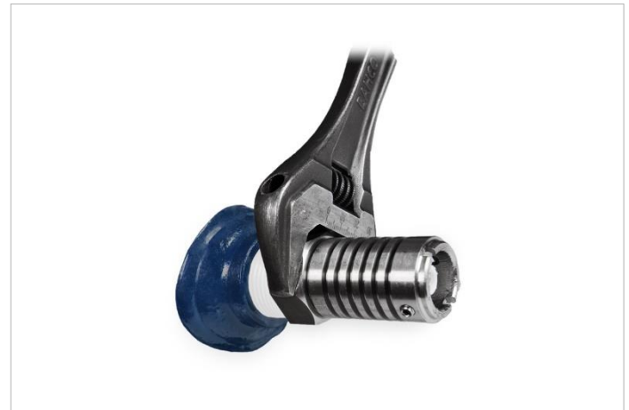
Fasten the mechanical part with a suitable spanner (tightening torque 80-150 Nm, depending on thread type).
