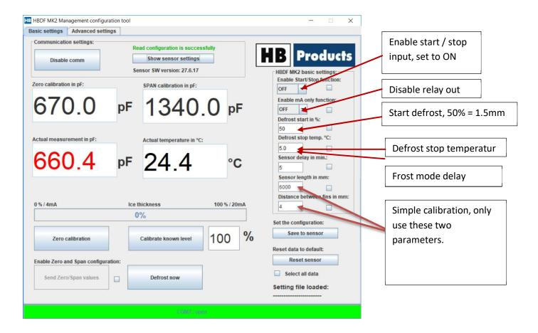
**Simple set-up**, only two parameters and execution of a zero/start point with frozen/dry evaporator surface (surface with thin layer of frozen ice as after defrost is the optimal start point). The length of the wire entered is only the wire between the fins, and not the free wire in the bending.
